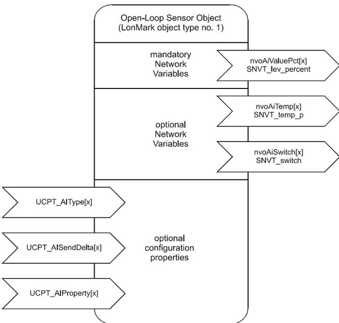
Fig. 2. Profile of LONMARK sensor object for UIs
