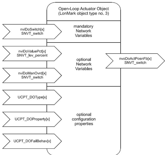
Figure 5. Profile of LONMARK actuator objects for relays
