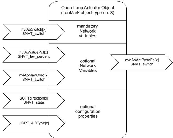
Fig. 4. Profile of LONMARK actuator objects for AOs
