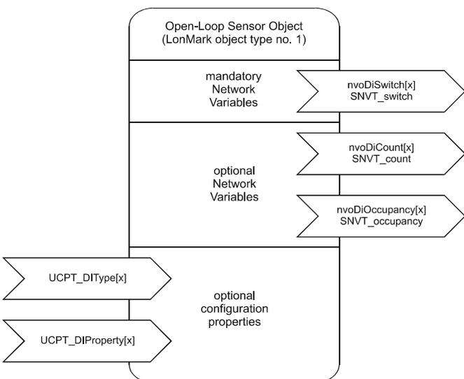
Fig. 3. Profile of LONMARK sensor objects for DIs
